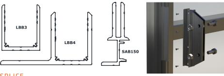
SAB150 must be fabricated into the mullions prior to installation. This allows attachment directly off the mullions through 2 purpose built holes.
